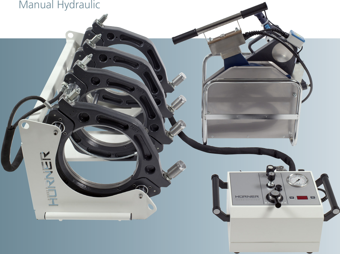
Stand-alone in Butt-Welding
